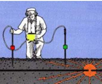
Ease and speed of fault finding with a thumper have been greatly enhanced with the addition of the S.D.A.D. to the Aqua-Tronics line. The Super DAD conveys more information about the fault location, and faster, with the addition of new microprocessor controlled electronics that provide bright, easier-to-see-and-read signals - day or night.
